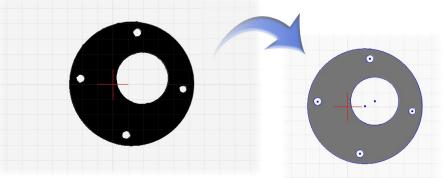
Comparison between scanned profile and reference CAD profile with overlapping and automatic centering
